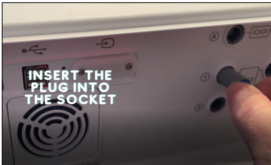
Figure 3: Connection between Sandman.IC and a medical device.
